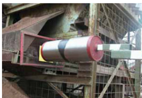
Lifting tool for changing conveyor feed
