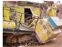
Damage to catwalk
