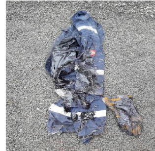
Bitumen covered PPE
