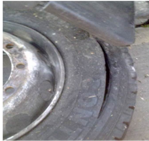
Tyre showing side wall failure
