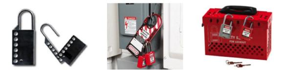
A hasp works by allowing each employee to attach their lock to the energy source. This means that a device or hasp is used to lock an energy source and then, in turn, each employee locks out the hasp. This ensures that the device cannot be removed from that energy source until all employees have removed their locks from the hasp. A hasp is required at each energy source for a lock out with multiple employees. Sufficient numbers, including spares, must be readily available.
