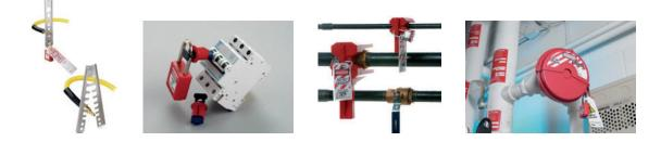
Lockout devices are items of equipment which, once put in place and locked off, prevent the operation and activation of switches, buttons, valves, and the reconnection of electrical circuits and hydraulic or pneumatic systems. They are generally used where the direct use of padlocks or hasps cannot be used to prevent activation/operation of the equipment. Once in place the lockout devices are then able to be padlocked/hasped as shown.
