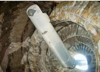
A high pressure, boom mounted, water nozzle is inserted through the back of the mixing drum. The nozzle is tilted close toward the back of the mixing blades for efficient cleaning.
