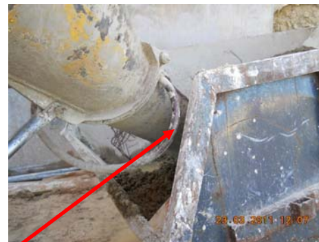
The nip point between skip and chute handle
