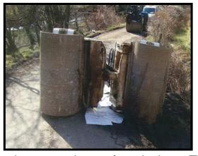
The operator was saved from serious injury due to two key safety devices. The seat belt prevented him from falling from the seat and underneath the roller – the ROPS (Roll Over Protection System) was in place protecting the machine from rolling completely over and protecting the operator's upper body and head
