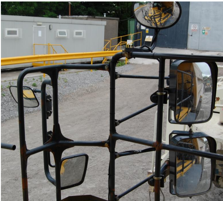
Typical mirror arrangement to achieve required Vision
