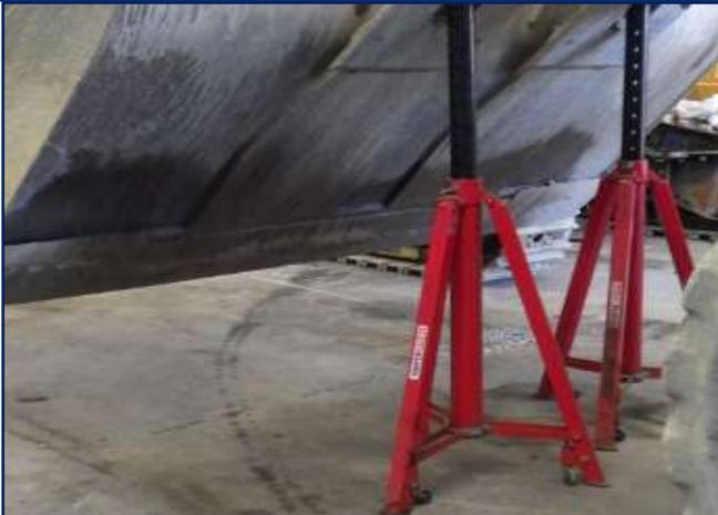
Axle stands, jack stands and any other equipment used to support the hydraulic attachment / arm, must be suitable for the job, in good condition and inspected pre-use. Any defective equipment should not be used.
