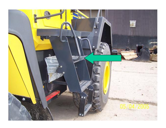
The minimum step angle of 15° was identified as being a key issue as the recommendation was to move away from ladders to true steps.
