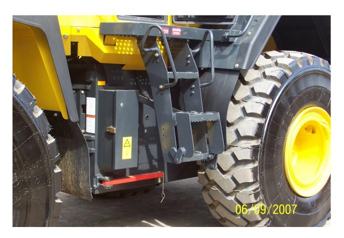
The Marubeni Komatsu solution was to fit a fixed bottom step that operated hydraulically via the ignition key. This step has a fail safe should the engine stop where it lowers automatically. An audible warning is also fitted at the customers request.
