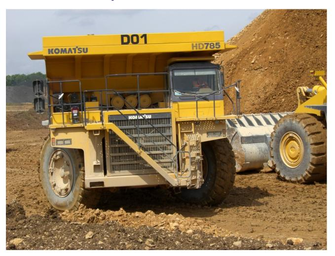
The bottom section of the steps fold up when the machine operates
