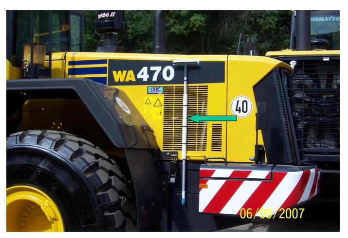
Fit an adjustable screen cleaner to the machine for ground level access
