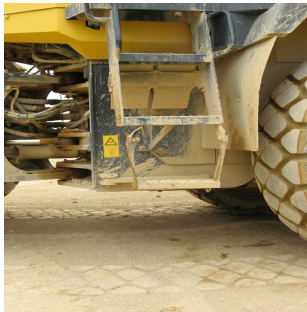
Steps leading down from loading shovel
