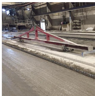
Chains on spreader beam
