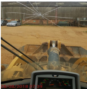
Crack on windscreen caused by impact with head
