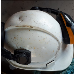
Hard hat with dent along back near centre
