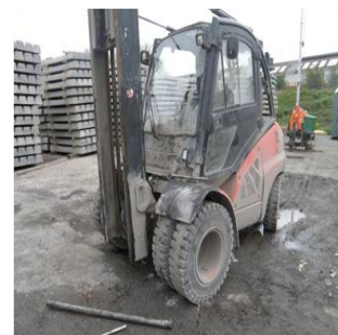
Fallen Mast Section
