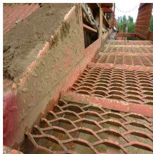
Meshwork walkway on Finlay 683 screener
