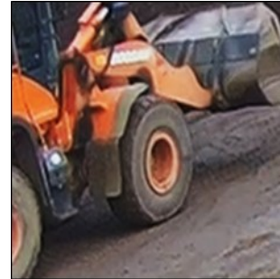
Tyre bulge prior to explosion
