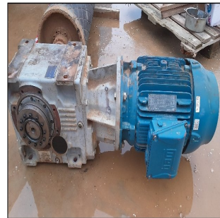
Motor and gearbox (eyebolt socket on motor)
