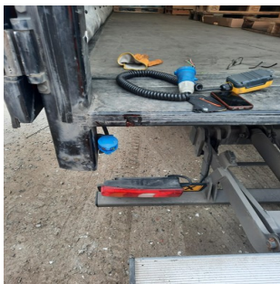
Rear of lorry and tailgate lift controller
