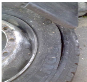
Tyre showing side wall failure
