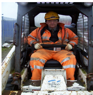
Operator wearing seatbelt, with isolator bar in position
