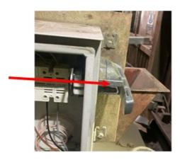
During a thorough investigation it was discovered that a square nut, which is intended to prevent the handle being depressed past its limit, had become loose and moved. This meant that the handle could be depressed further than intended, this allowed the padlock to 'slip' off.
