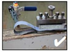
The tool post is used to clamp and hold a looped strip of emery cloth in place during application. (see video demonstration).
