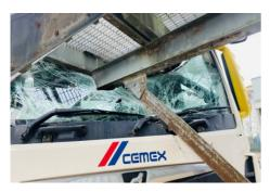
Fortunately, the driver was unharmed; however, the staircase penetrated the vehicle cab, which could have potentially caused serious injuries.
