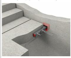
Invisible Connections has developed a system for the installation of precast stairways and landings that significantly reduces these risks based on telescopic connectors.
