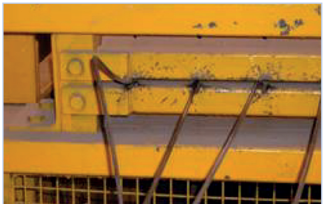
Figure 4.21 Wire/strand kinked on stressing bed.
