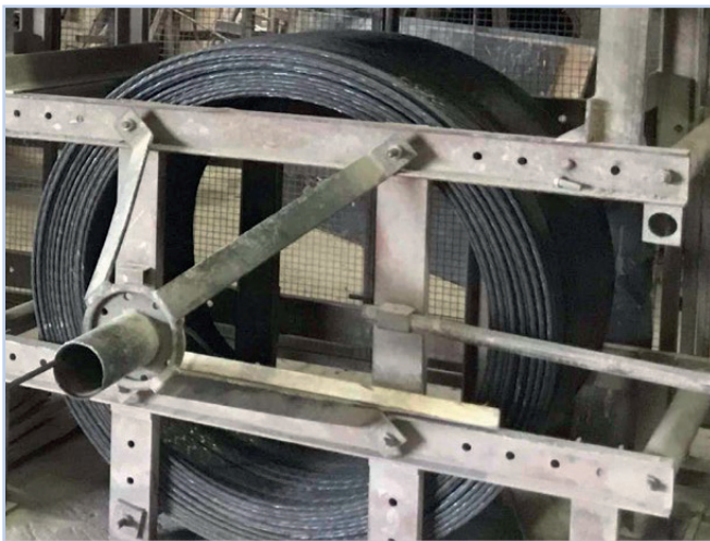
Figure 4.19 Strand dispenser with extended nose to help prevent tangling.
