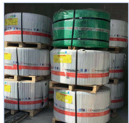
Figure 4.7 Strand coil laid 'eye to the sky'.
