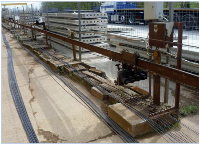
Figure 5.4 Rabbit mechanism on raised track for pulling pre-determined lengths of wire/strand.
