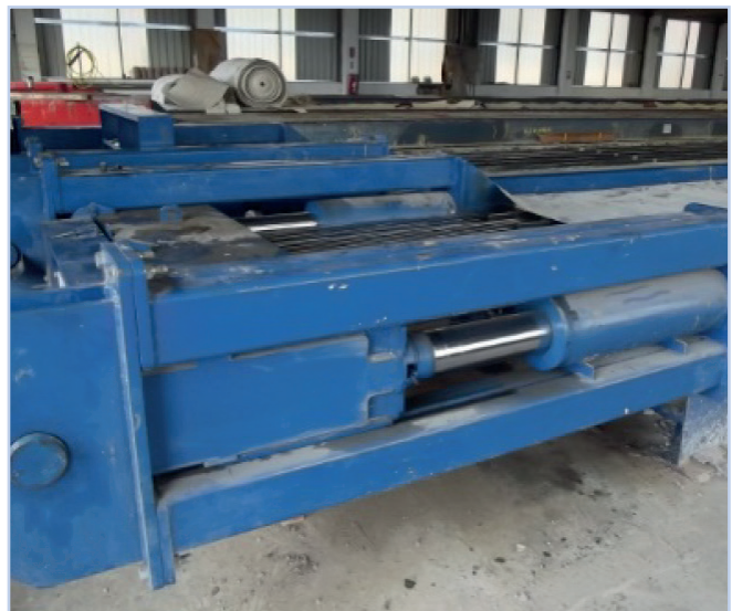
Figure 7.3 Multi-stressing mould in tensioned position.
