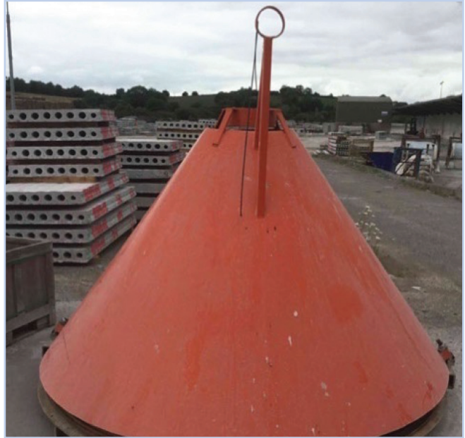
Figure 4.12 Cover lifted by forklift truck protecting wire from the elements.
