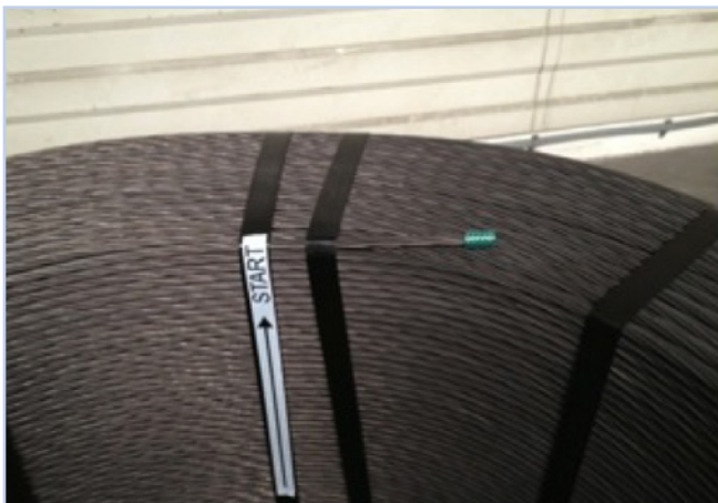
Figure 4.23 Coils of strand showing indications of where to start pulling.
