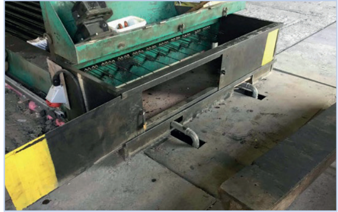
Figure 7.21 Sliding cover used to enclose stressed wires.
