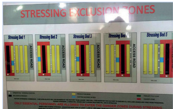
Figure 7.22 Example of stressing exclusion zones.
