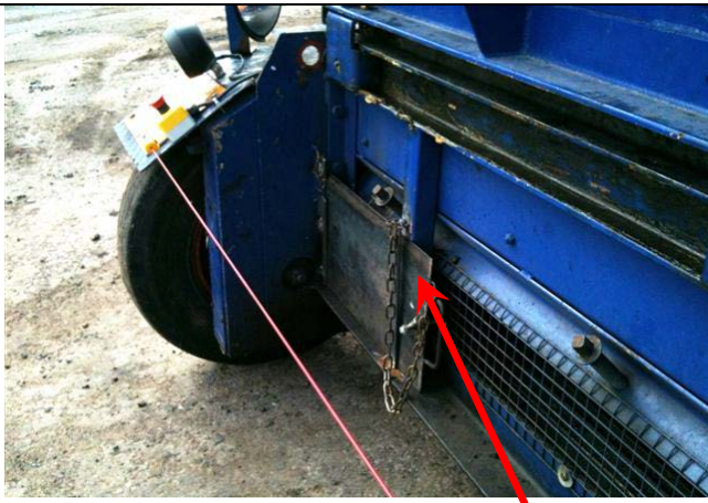
External Blanking plate secured to front of chipper
