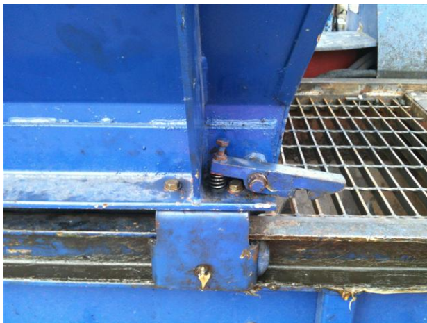
Sprung hopper catches to secure catches in place and prevent accident release whilst in transit
