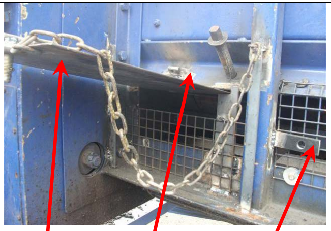
Blanking plate being inserted
