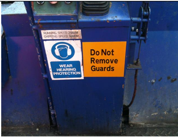
Example of warning signs to be fitted
