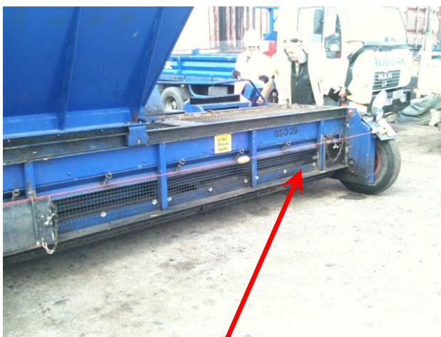
Mesh guarding to be fitted across the full width of the chipper to prevent access to moving parts
