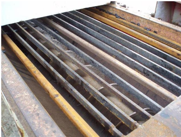
Open parallel bar or mesh guarding which extends the full width of the chipper hopper
