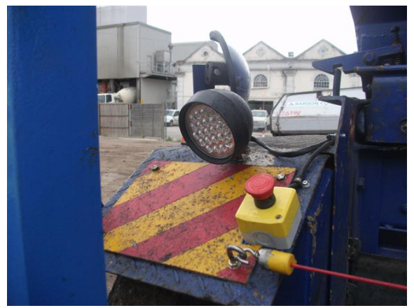
LED lights fitted to either side of the machine, to give improved visibility for night working
