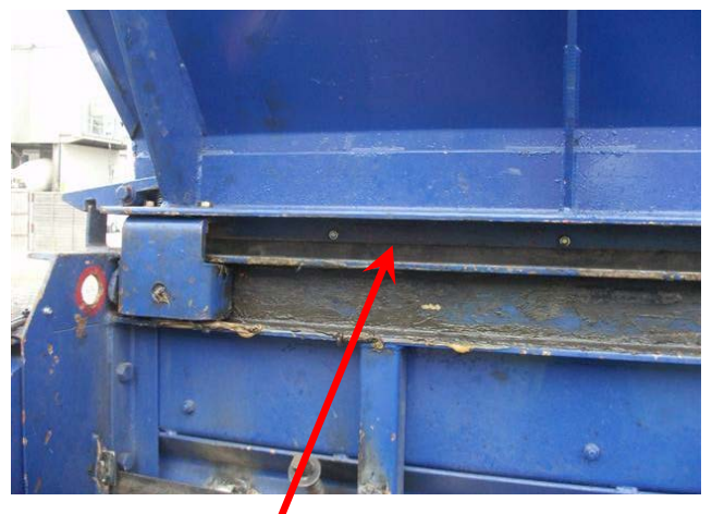
Rubber skirt fitted to the bottom of the hopper to reduce the potential of spillage
