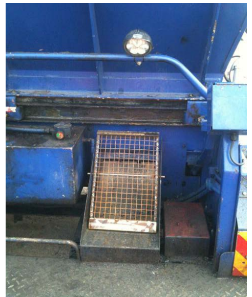
LED lights fitted to either side of the machine to illuminate the 'chipping up' access chute(s)
