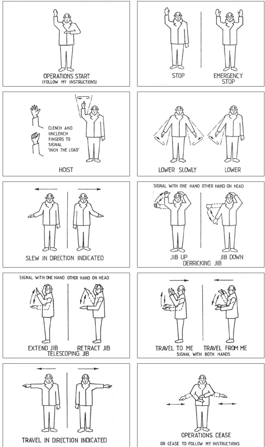
Figure 10.6 Recommended crane signals
