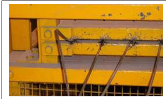
Figure 3.20 Wire/strand kinked on stressing bed
