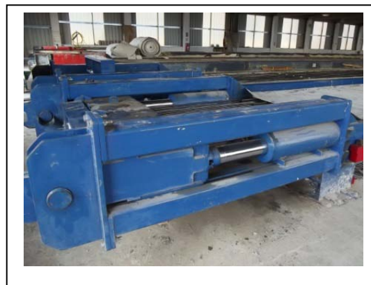
Figure 6.3 Multi-stressing mould in tensioned position. Arrow indicates direction of pull
