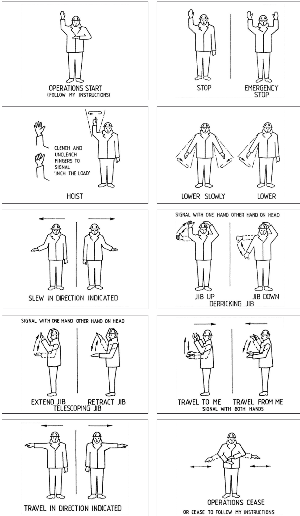
Figure 10.6 Recommended crane signals
