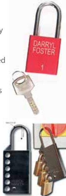
**Hasps** – Multi hasps are used when multiple individuals are involved with an isolation and are accountable for their own safety. The function of the device means the energy can't be restored until all padlocks are removed from the multi hasp.
