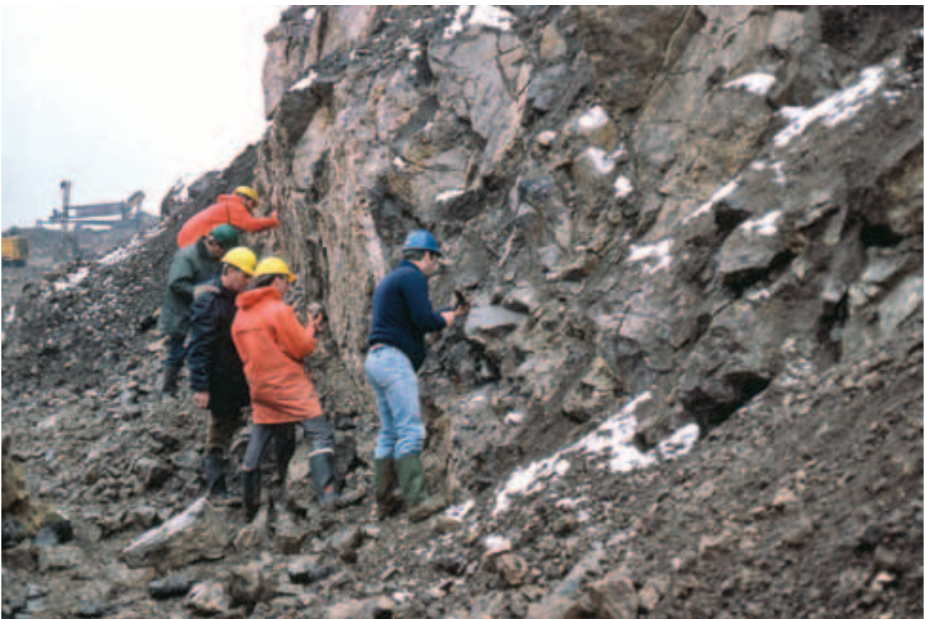
Fluorspar openpit operation, Dirlow Rake, Castleton, Derbyshire. Visitors collecting samples of fluorite minerals. Although the face is quite low there is a significant hazard from rockfalls. The visitors are not wearing high visibility vests or jackets as there was no legal requirement for this when the photograph was taken in the early 1980s.
