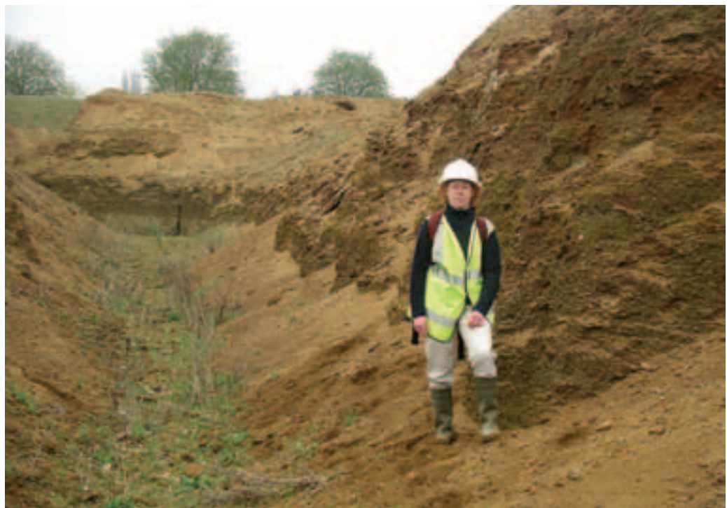
A visitor to an active quarry wearing appropriate personal protective equipment. The quarry face is away from the active working area, is stable and direct access presents an acceptable risk to the visitor. The site is extremely important for its geology as it is the best of only three where these strata are exposed. Faringdon Sponge Gravels, Wicklesham Quarry, Oxfordshire.
