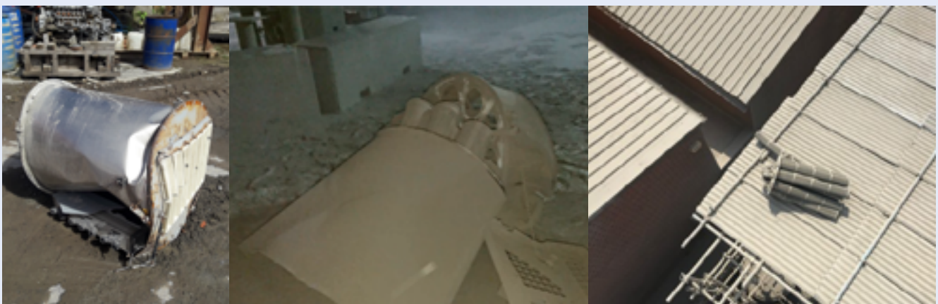
An over-pressurisation incident lead to the 'launching' of this filter housing from the top of a silo. If this had landed on anyone, they would have been killed.
