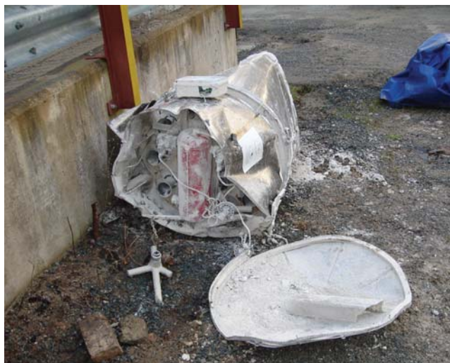
Figure 7 Filter Housing which has been ejected from the top of a silo
