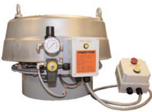
Figure 4 Pressure relief valve with test facility (which is claimed to be able to test the valve from ground level before delivery commences and to facilitate cleaning of the valve without requiring dismantling).
