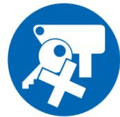
**Remove all keys** to ensure a vehicle cannot be started without the isolators knowledge. Follow the steps of LOTOTO for full isolation. If a removable isolation brake key is available, ensure this is removed as a part of the isolation process.
